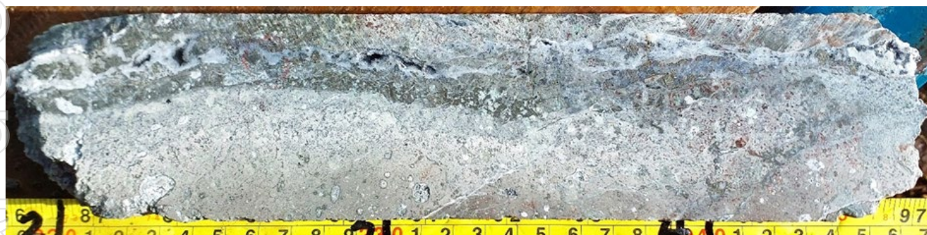
25VDD002_199.58-199.83m. From Sample No. 386656, 199.32-199.9m (0.58m), 26.4 g/t Au, 39.70 g/t Ag. Colloform banded and crustiform chalcedonic silica veins. Open spaces with drusy quartz. Blebby and fine pyrite, sphalerite and galena-tennantite-tetrahedrite. The host lithology is a vesicular basalt and silica-clay-altered. Disseminated and bebbpy pyrite halo to the veins.
