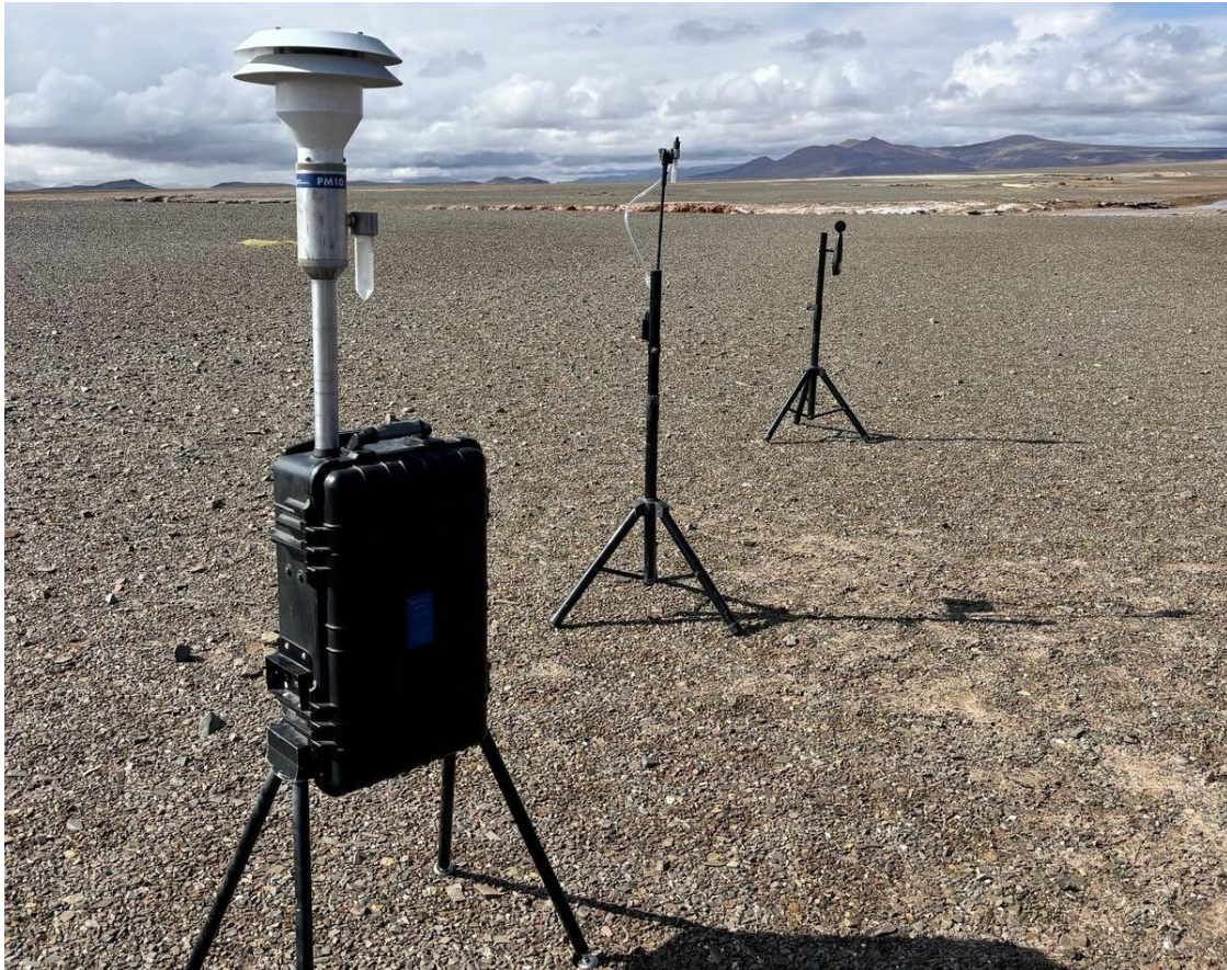
Figure 9. Air and sound monitoring equipment employed near drill hole JAM 24-03
