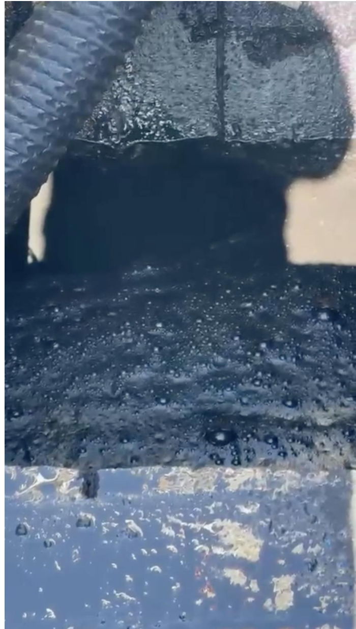
Figure 1: Photo of visible gas observed from drilling mud taken along the length of targeted seam IIIb
