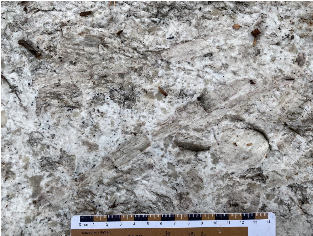
Figure 4: Large, light grey spodumene crystals at the CV15 Pegmatite in a matrix of feldspar, smoky quartz, and minor mafics.
