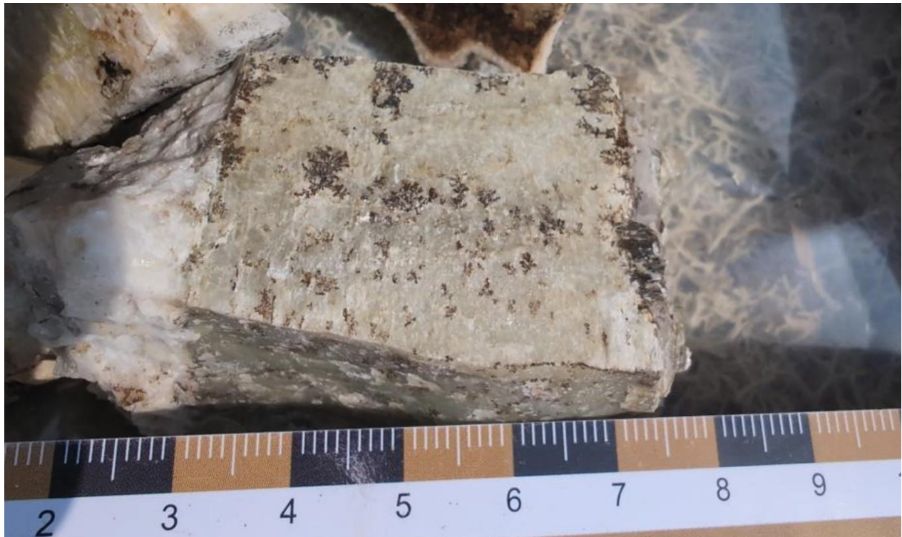
Figure 8: Light green spodumene crystals in a matrix of feldspar and smoky quartz from angular boulder (0.93% \text{Li}_2\text{O} ), located northwest of CV5.
