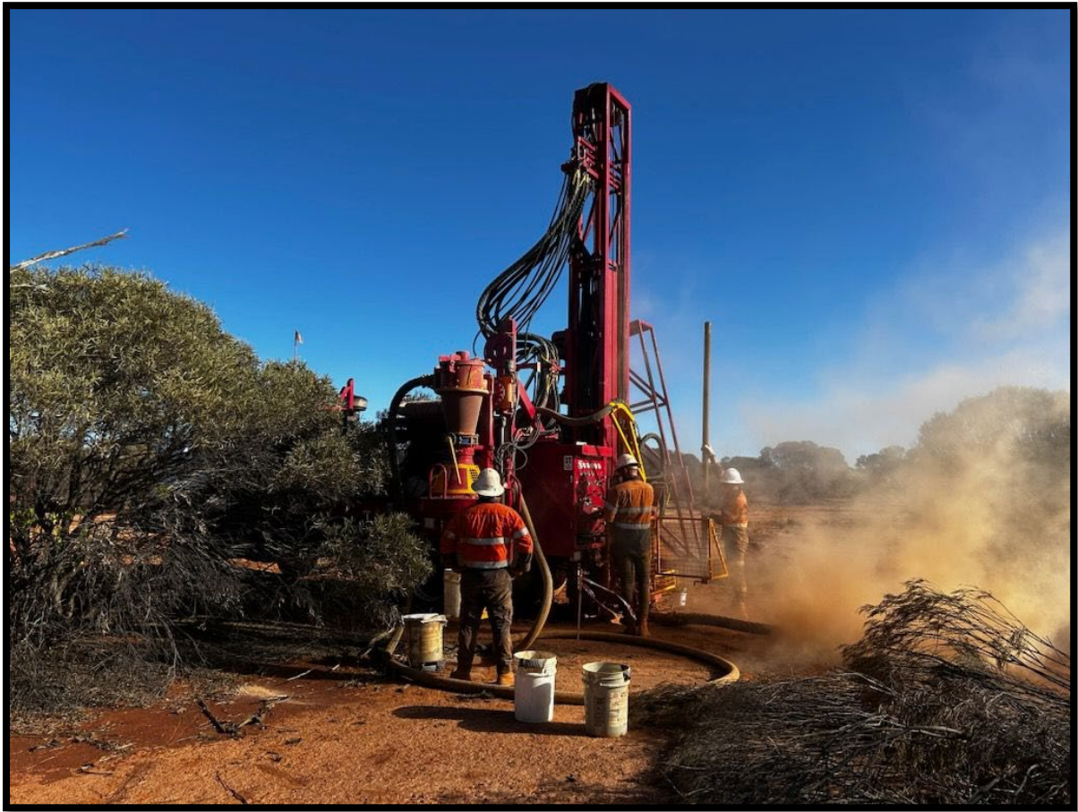
Figure 1: Fenceline aircore drilling in progress at Revere
