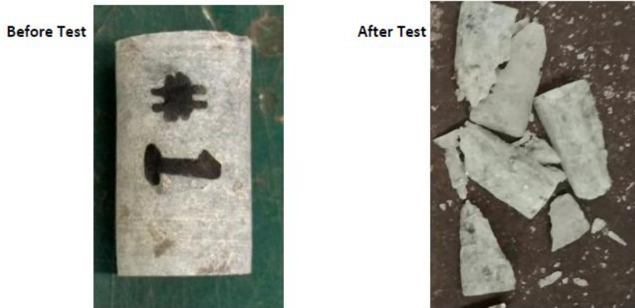
Figure 4 – Before and after UCS testing on sample WCDDMET012_1
