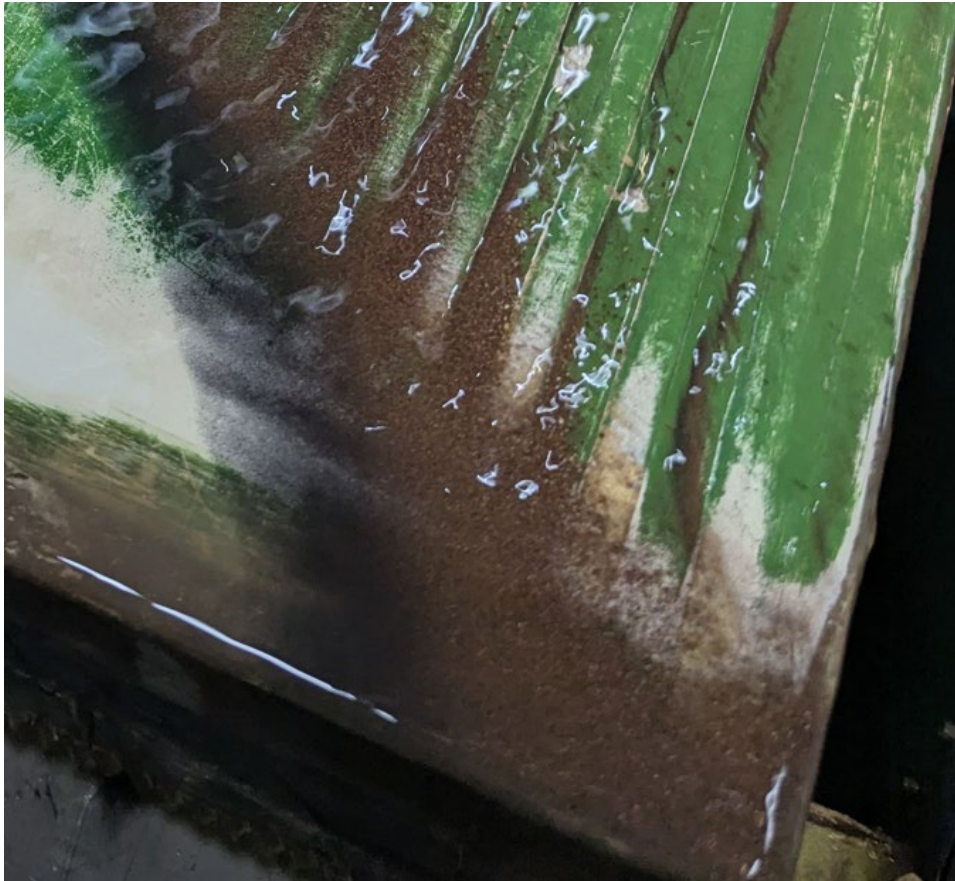
Figure 1: Shaking table test work distinct mineral banding highlights excellent gravity separation potential of the Mata da Corda ore.
