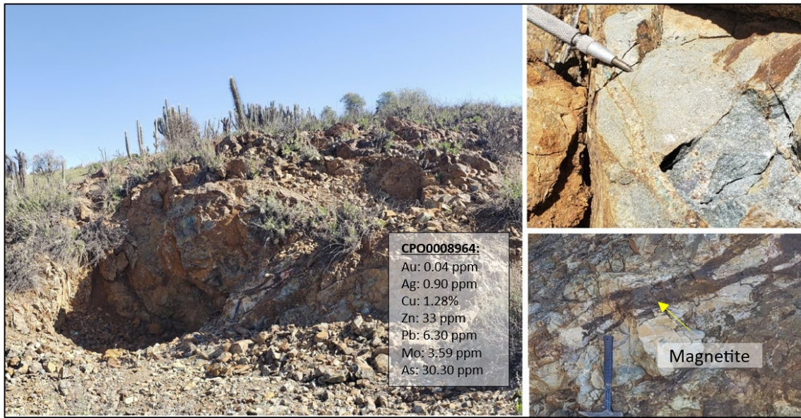
Figure 9: Sample CPO0008964 - Andesite host rock, brecciated texture with chlorite-epidote-albite alteration, featuring mineralisation in vugs and patchy zones with limonite, copper oxide, and magnetite. 22,31
