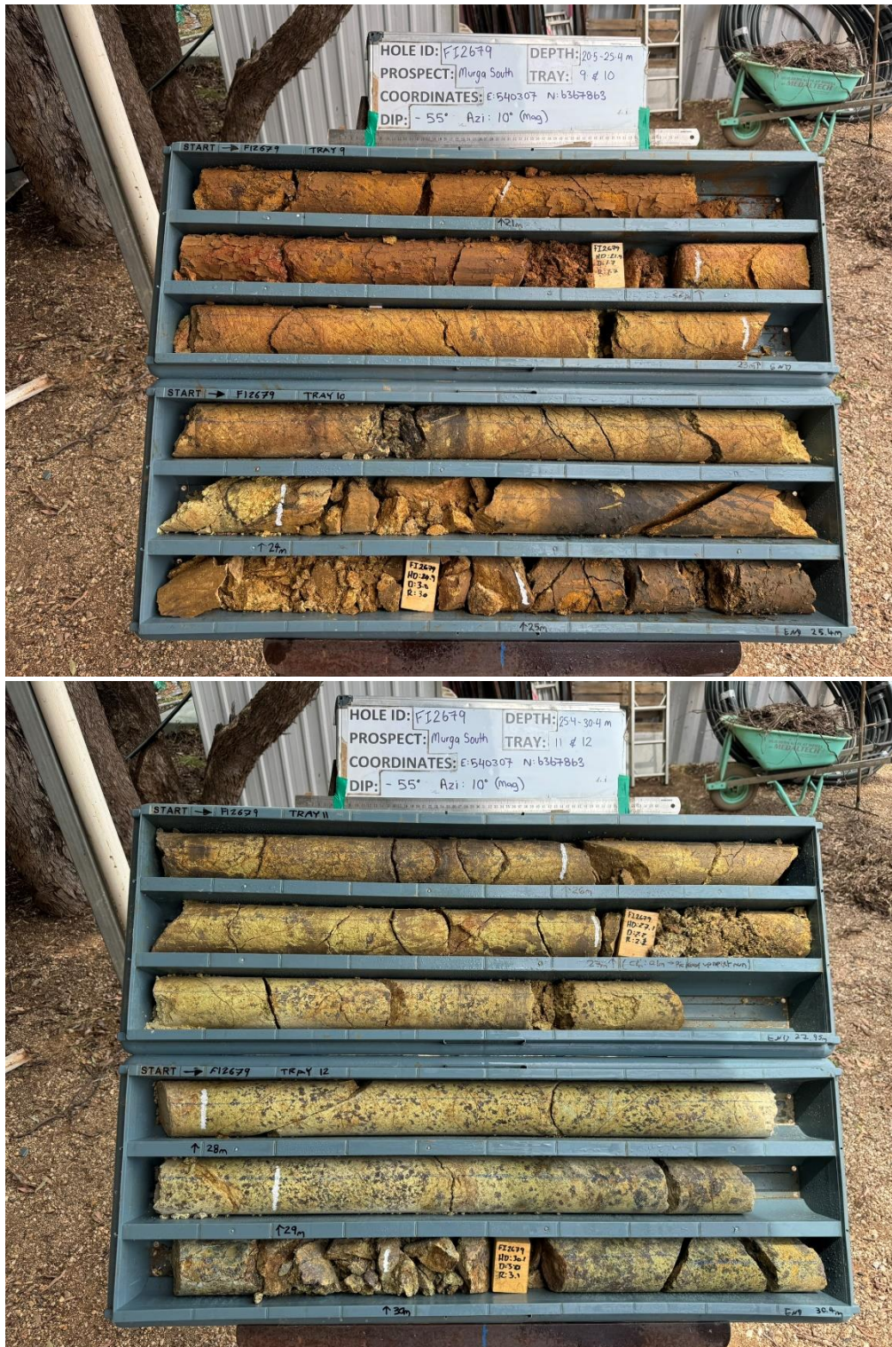
Figure 5c: F12679 – photos of diamond drill core 20.5 to 30.4 metres (laterite / lower saprolite)
