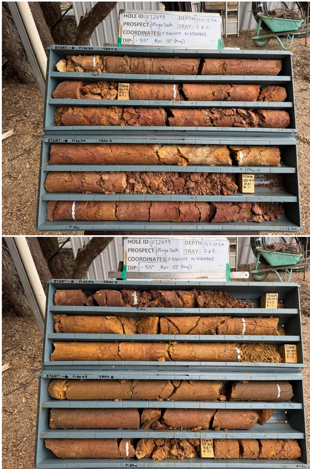
Figure 5b: FI2679 – photos of diamond drill core 10.5 to 20.5 metres (laterite zone)
