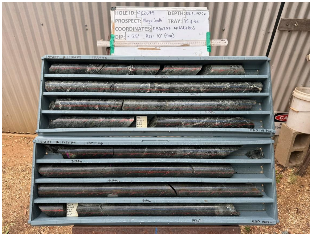
Figure 6a: FI2679 – photos of diamond drill core 135.5 to 142.2 metres (lower Sc enriched pyroxenite zone)
