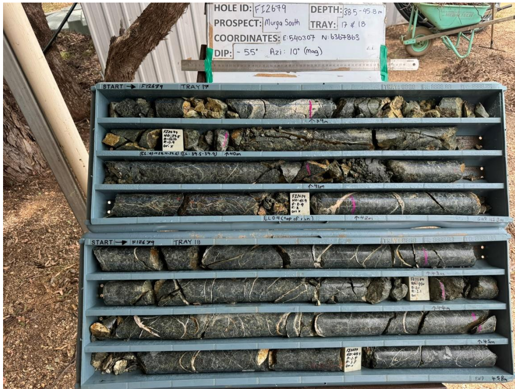
Figure 5e: FI2679 – photos of diamond drill core 38.5 to 45.8 metres (fresh rock)
