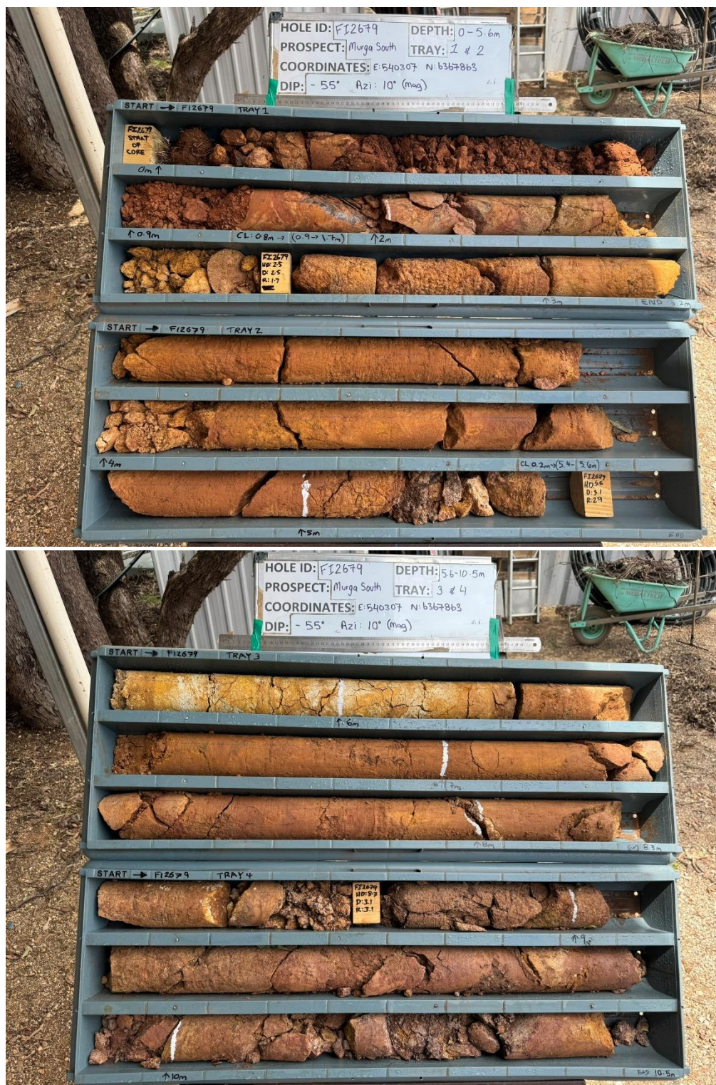
Figure 5a: FI2679 – photos of diamond drill core 0 to 10.5 metres (laterite zone)
