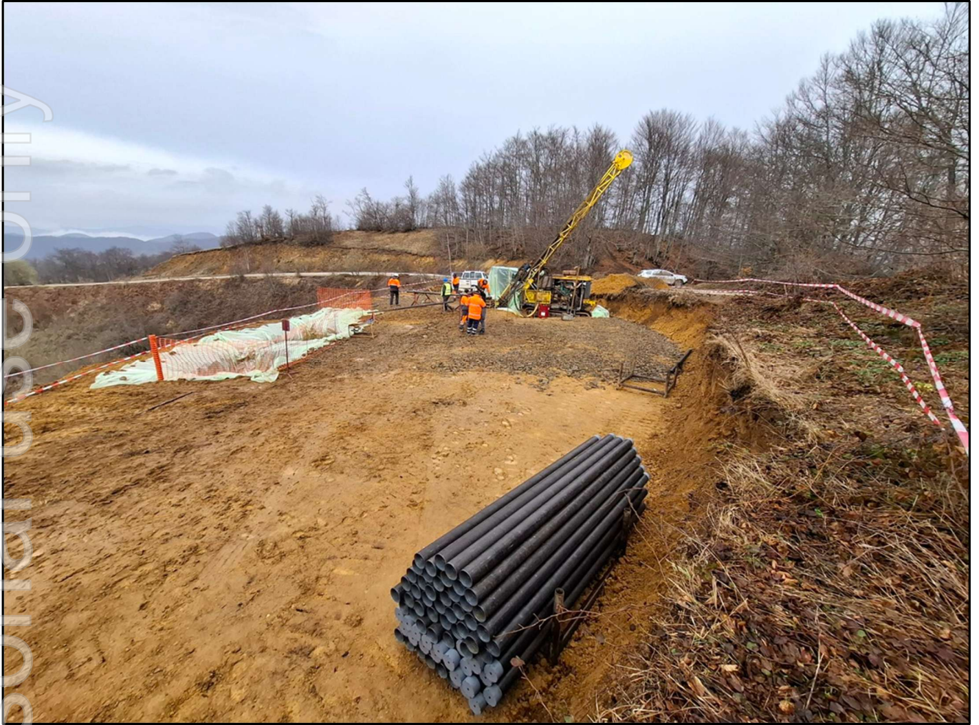
Figure 2. Photo of the fifth diamond rig set-up at Obradov Potok.
