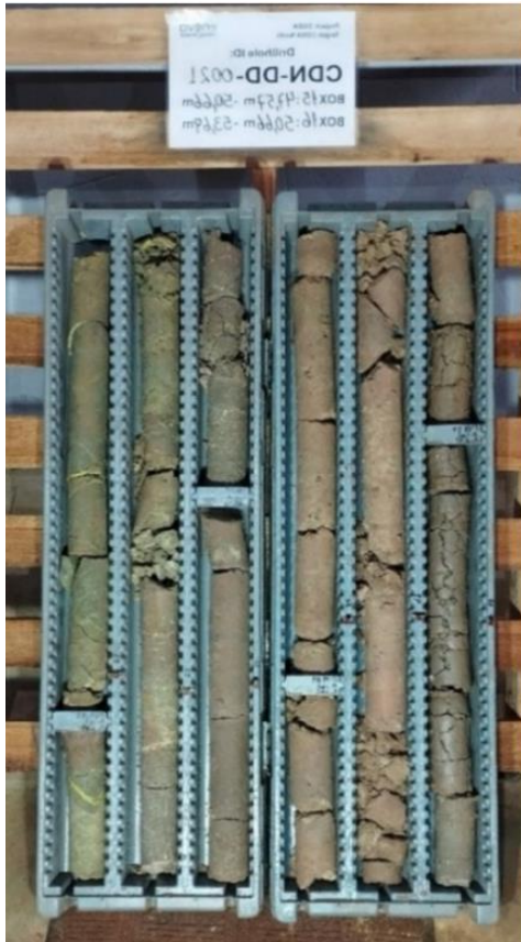
Figure 3: Diamond drill core within saprolite and saprock representing kamafugite litho-unit.
