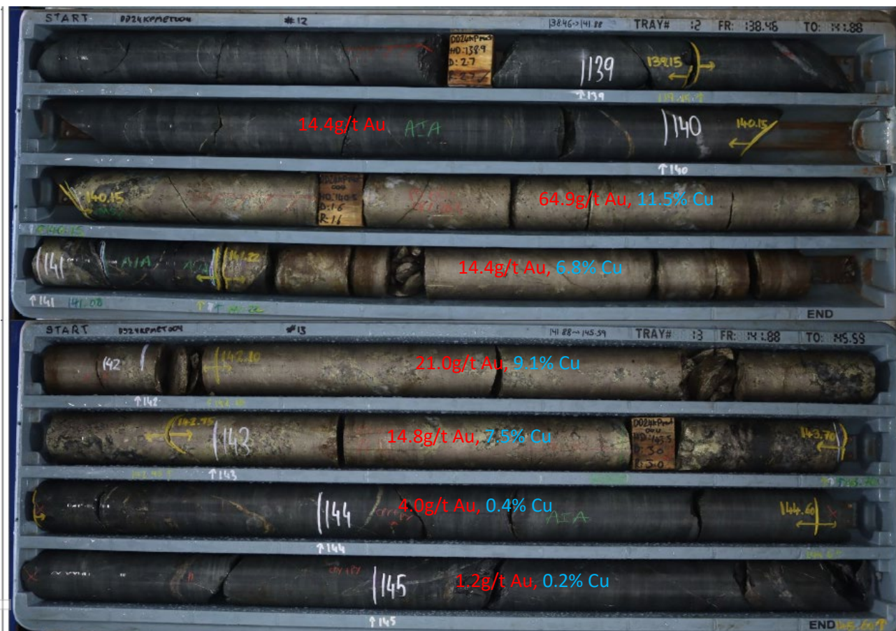
Figure 2: DD24KPMET004 semi-massive to massive sulphide (pyrite and chalcopyrite) vein hosted in andesitic host with 2-10mm quartz-sulphide (pyrite and chalcopyrite) veinlets. Sample intervals marked in yellow. Gold (red) and copper (blue) grade detailed for each interval included in the significant intercept.
