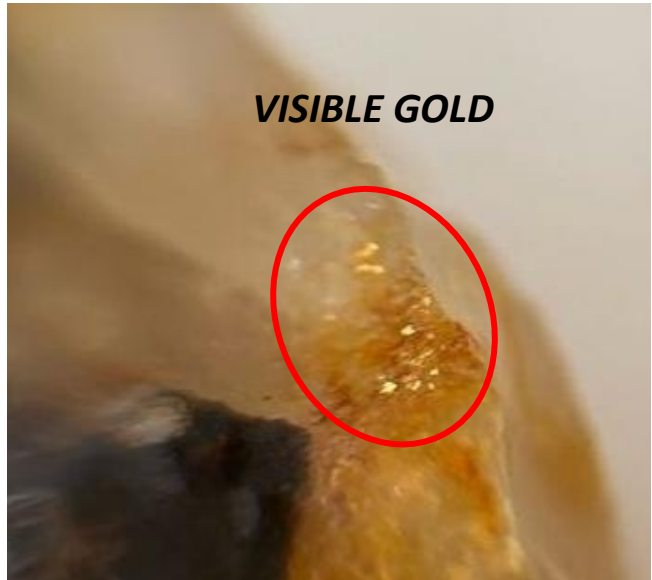
Photo 1: Visible gold observed in drill hole NMWBAC25-897: 41-42 metres. Returned a composite gold grade of 4 metres @ 2.8 g/t Au (within 8 metres @ 1.47 g/t Au) from 40 metres
