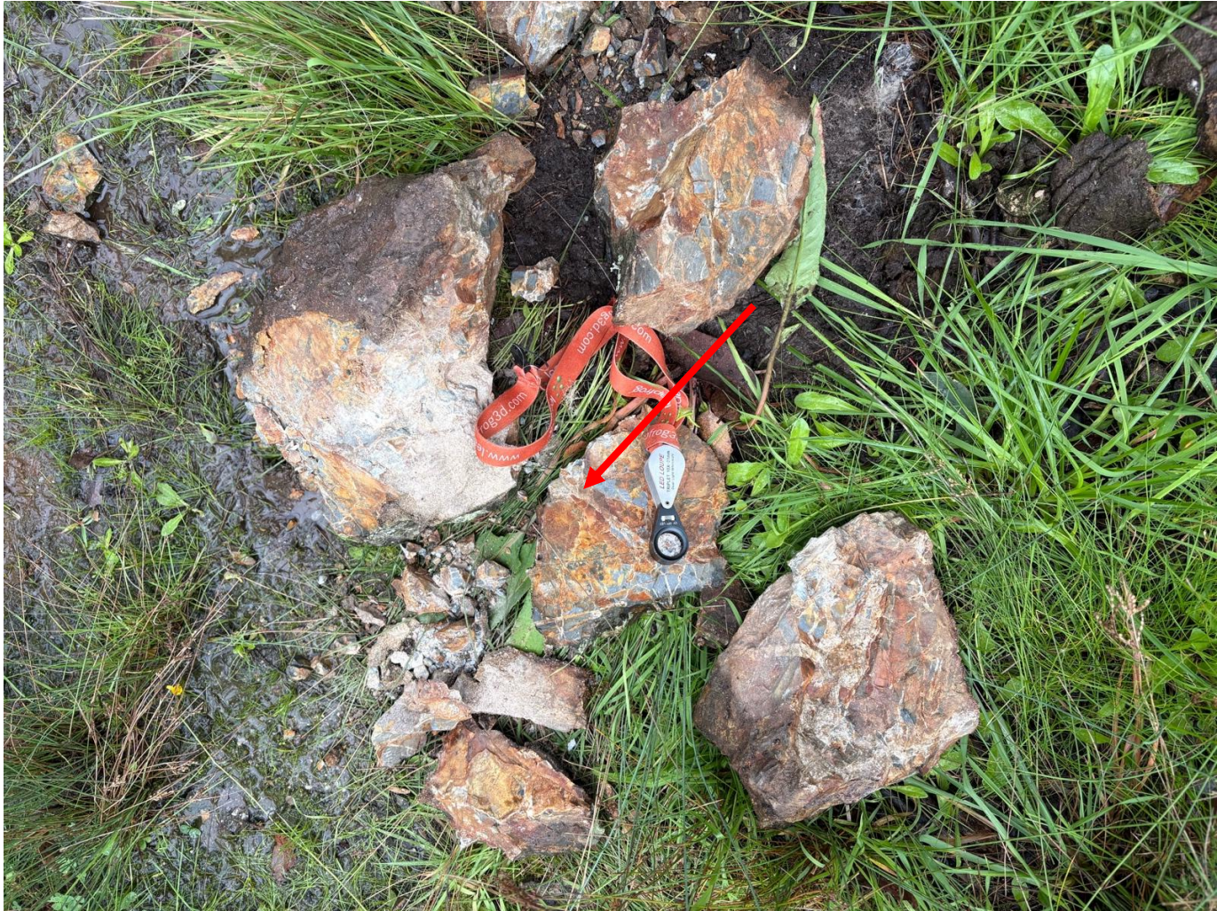
Figure 3. Quartz breccia sampled from dump material at the Achill Prospect, Rockvale Project (disseminated stibnite observed, visual estimate of 1-2%)
