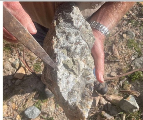
Figure 5: Hand specimen of brecciated, silica-flooded, sulphidic rock at Mountain Maid.
