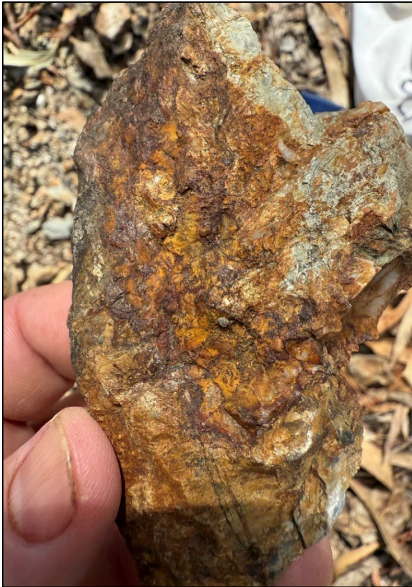
Figure 3 – Gold mineralisation within ferruginous shale and quartz yielding 82.7 g/t Au from sample 3001464
