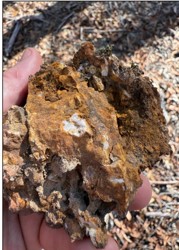
Figure 4 – Gold mineralisation within ferruginous quartz vein yielding 82.1 g/t Au from sample 3001379
