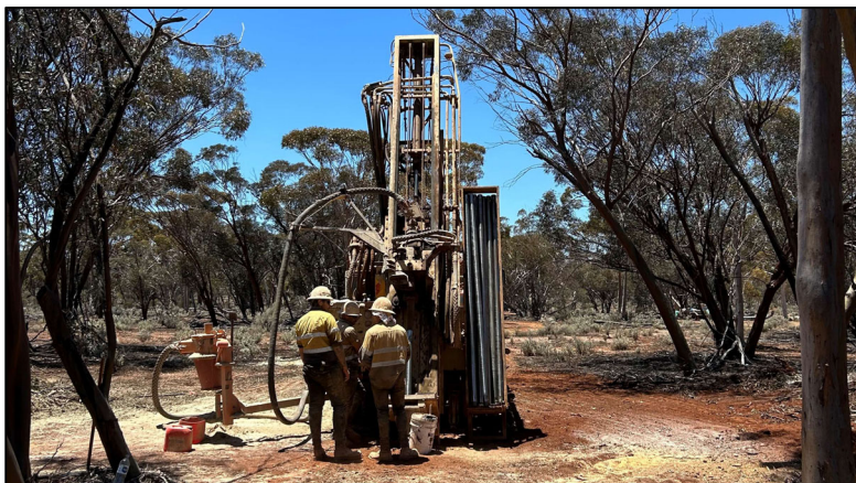
ASQ 2024 Aircore Drilling at Golden Wishbone
