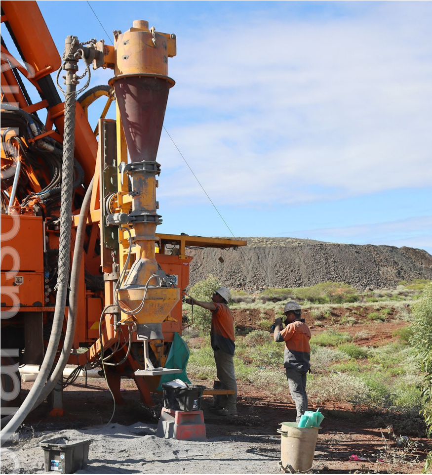
Photo 1. Running in the Gyro for a downhole survey.
