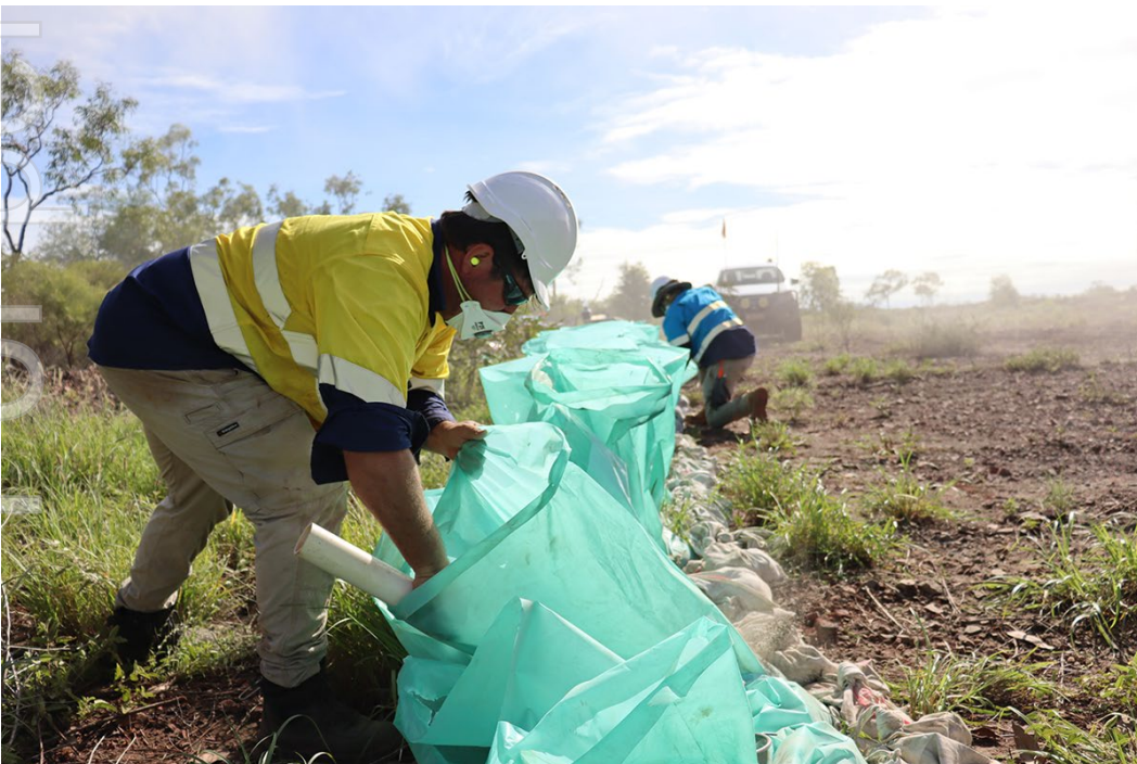
Photo 2. Spearing sample with PVC for the geological chip logging.
