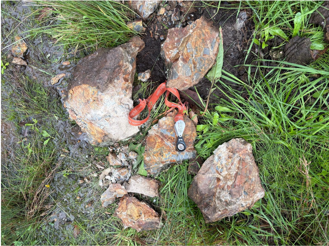
Figure 3. Quartz breccia sampled from dump material at the Achill Prospect, Rockvale Project (disseminated stibnite observed, visual estimate of 1-2%) – See table below for further details of sample shown above.
