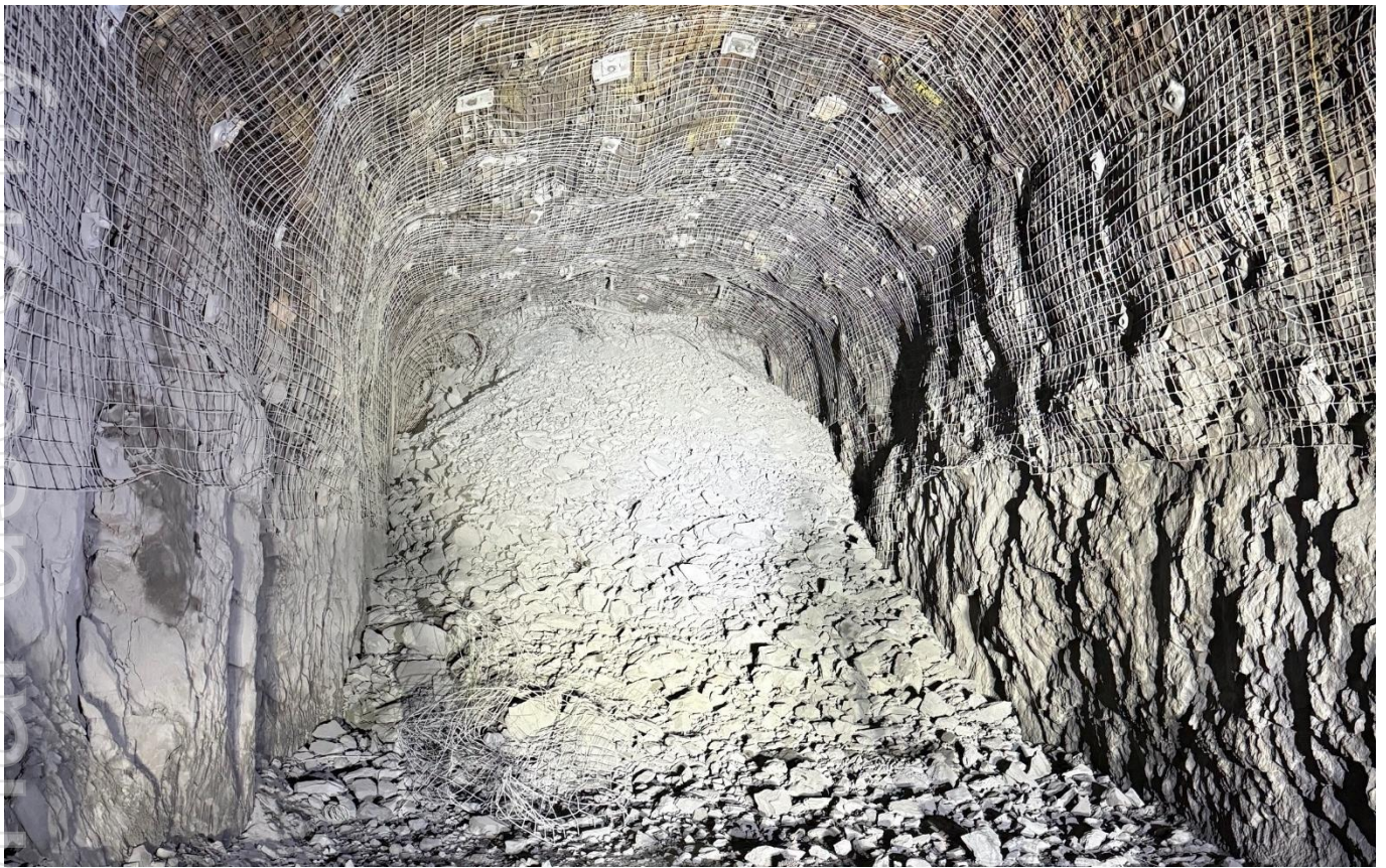
Figure 2: First stope blast on the 775 level – Diluted block grade 180g/t Ag, 6% Zn & 3.8% Pb.
