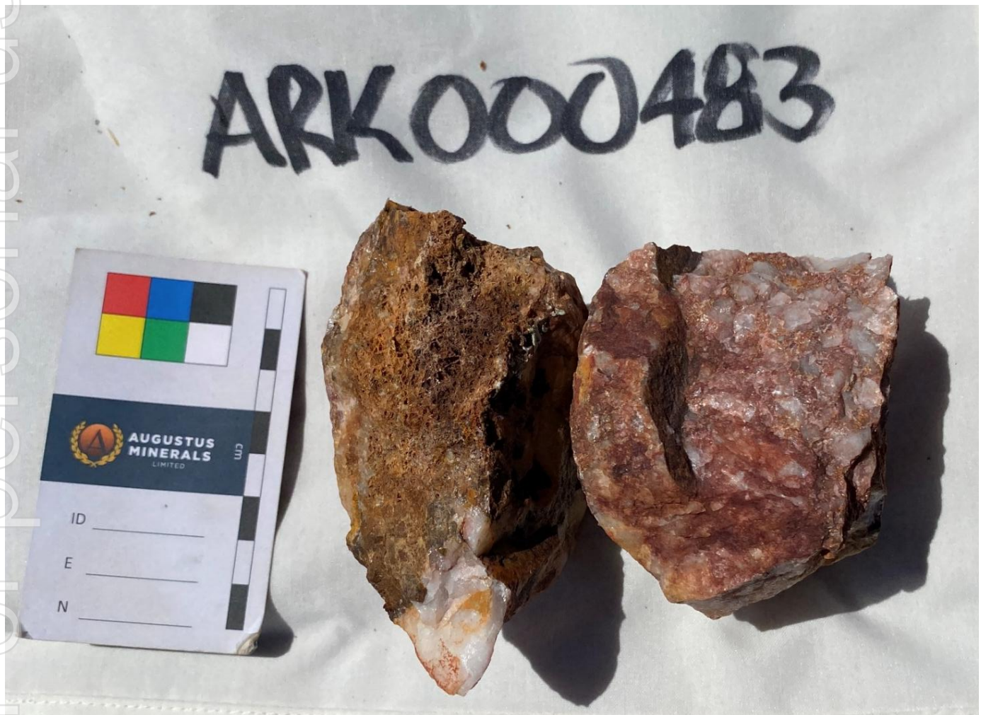
Figure 11 Rainbow gossanous quartz vein which assayed 75g/t Ag with strongly anomalous Bi to 114ppm and Te to 44ppm (sample ARK000483).
