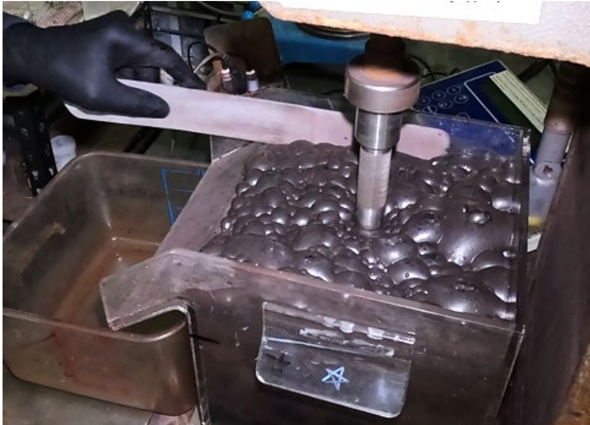
Figure 2 - Bench scale flotation testwork at Bureau Veritas laboratories, Adelaide
