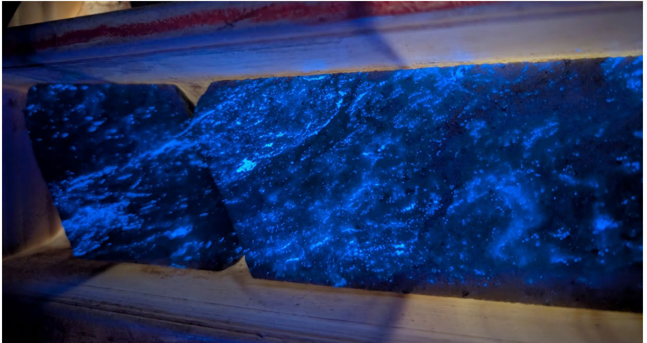
Figure 1 – WQSDD002 from 172-173m grading 2.49% WO 3 under UV light
