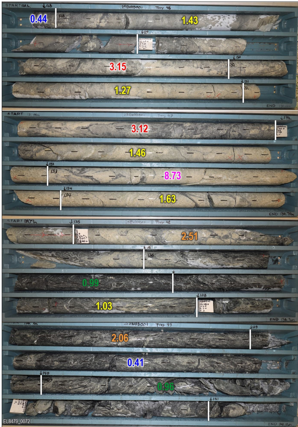
Photo 3. Core tray photos of 25ENDD001 interval 16m @ 2.14g/t Au from 128m (part thereof).
