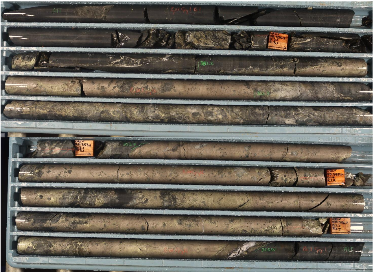
Figure 6: DD24KP1232 - ~6.65m interval of massive and semi massive sulphides overprinting quartz veining from 351.2m, comprised of pyrrhotite (60%) and semi massive chalcocopyrite (15%) and pyrite (5%). True width of the interval is estimated to be approximately 65% of the visually logged intercept length based on. Refer to Annexure 4 for further information about orientation of data relative to geological structure.
