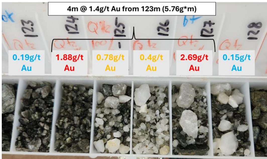
Figure 3: Chip tray from SRRC048 (123–127m), representing a 4m interval of footwall-hosted gold mineralisation. This zone supports the interpretation of a second stacked lode beneath the main shear. Note the quartz–biotite–pyrite veining within amphibolite, characteristic of the observed hydrothermal alteration.
