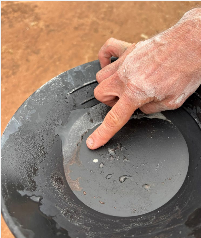
Figure 2. (Left) Panning of cassiterite (grains of dark grey to black material). (Above right) Collected cassiterite grains, sourced from BRC004 (108m, 7.99% Sn).
