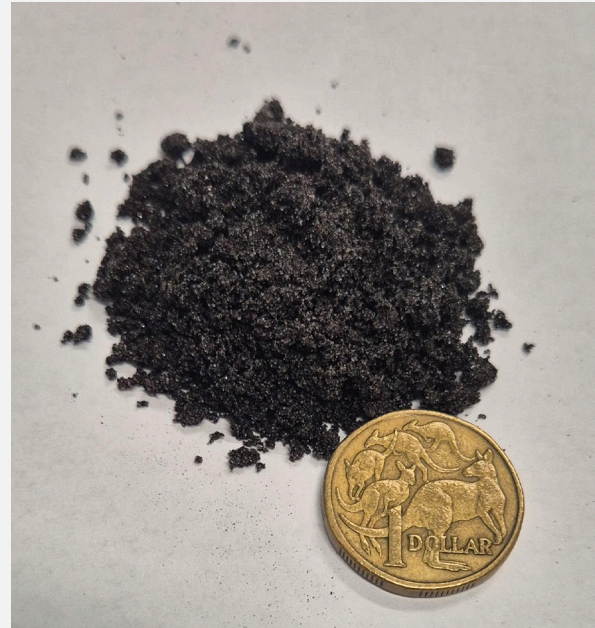
Figure 2. (Left) Panning of cassiterite (grains of dark grey to black material). (Above right) Collected cassiterite grains, sourced from BRC004 (108m, 7.99% Sn).
