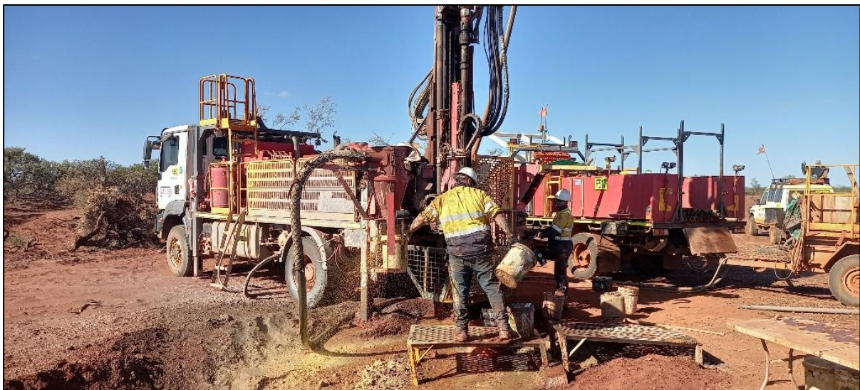
Figure 7. Operating Wallis Aircore rig
