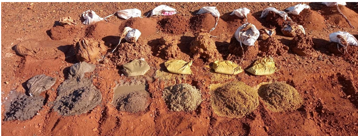
Figure 4. 24YRAC048 Aircore drilling samples showing mineralised redox boundary over the 60-66m interval grading from brown reduced carbonaceous sands down into bright yellow oxidised sands. Mineralisation occurs on the reduced side of the redox boundary
