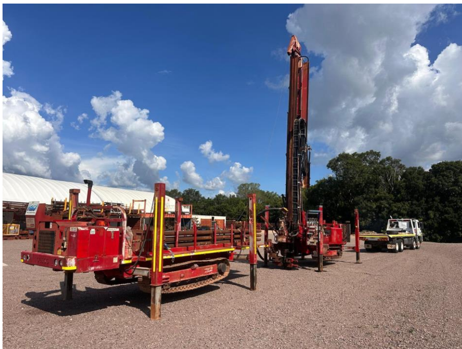
Figure 1: CoreSearch Rig 1 - SP6500 SA-RC-MP capable of both diamond and reverse circulation drilling along with one of two carriers containing two full rod strings and additional downhole equipment.
