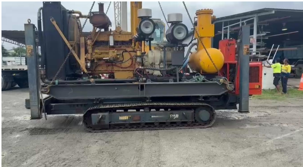
Figure 2: The Ingersoll Rand 1070/350 compressor mounted on the additional track carrier.
