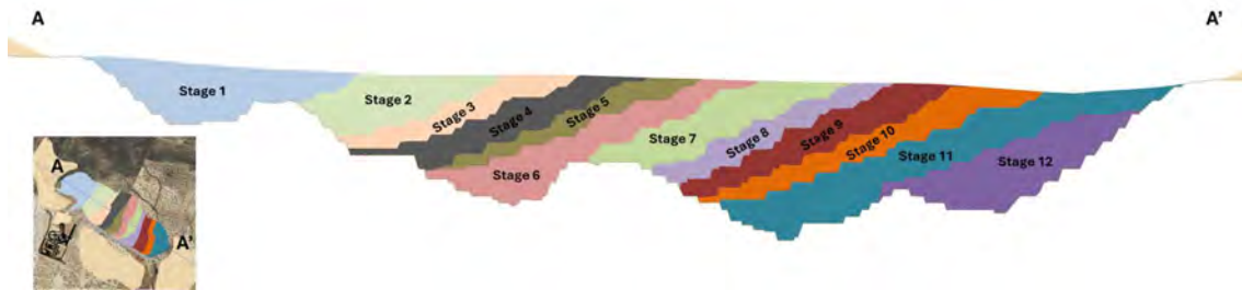
Figure 7-4 – DFS Pit Long Section Showing Mining Stages
