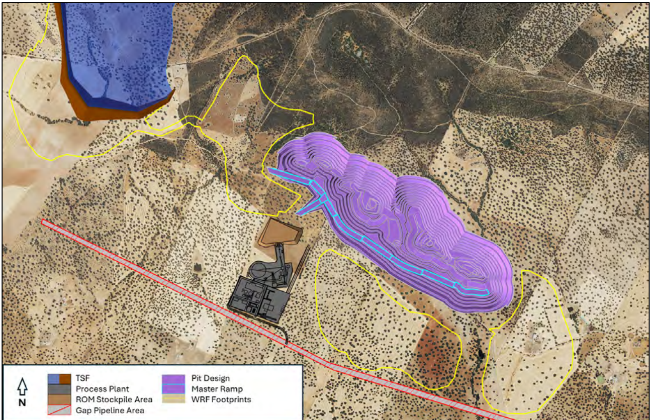
Figure 5-11: Layout of Mine and Infrastructure
