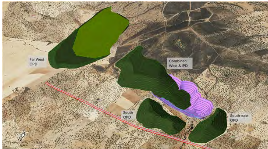
Figure 7-18 – Final Landform of Rehabilitated WRF and TSF
