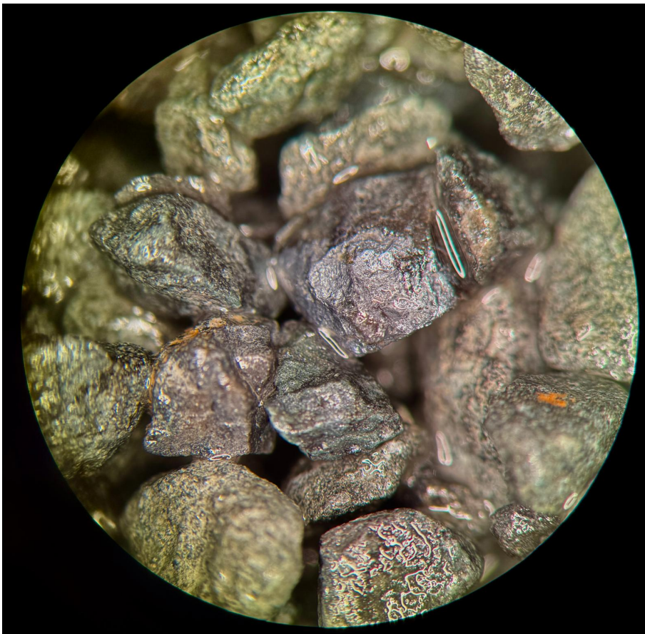
Figure 4. Chalcocite rich chips from DAN25003 between 69-70.5m depth.
