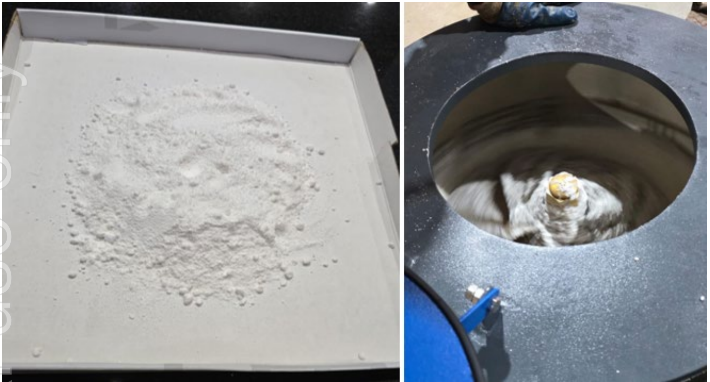
Figure 2 – 98.9% Lithium Carbonate (left) and processing in the plant's centrifuge (right)
