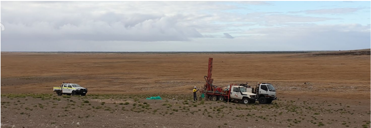
Figure 3: An example of low impact air-core drilling on the Eyre Peninsula to be utilised by CR3 at the Cummins Project.
