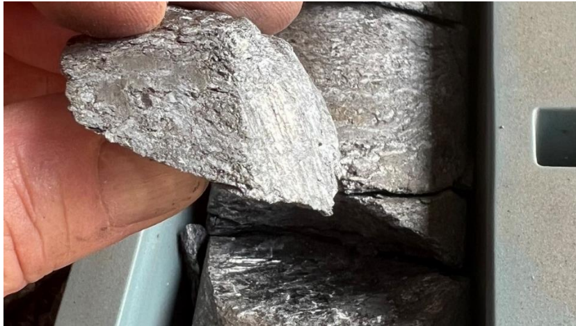
Figure 6: Graphitic Schist from LEDD_3 at 18.5m (interval 18-19m assayed 11.3% TGC)
