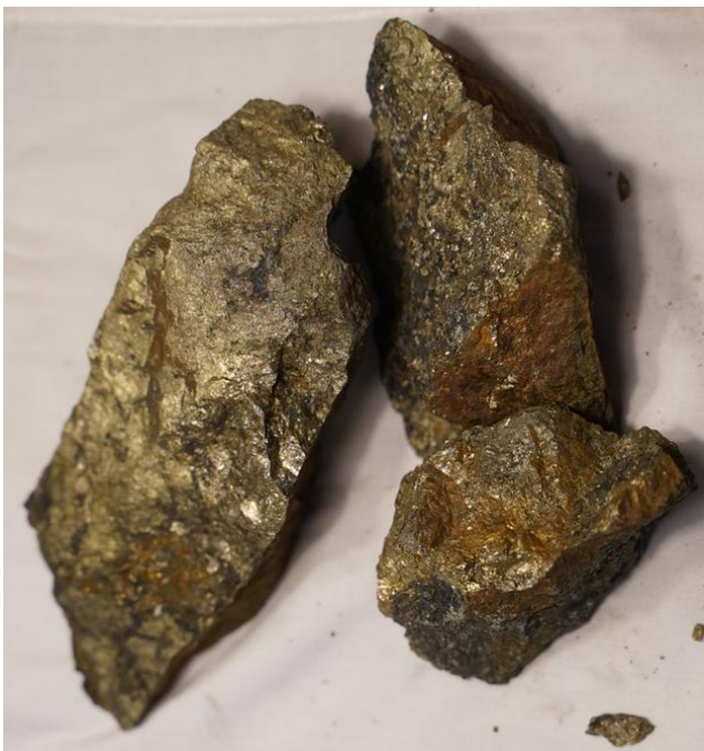
Figure 1: Prince Of Wales prospect sample RK008302 10.15% Cu and 65.8g/t Ag 2 , being tested for Induced Polarisation, chargeability, galvanic resistivity and inductive conductivity
