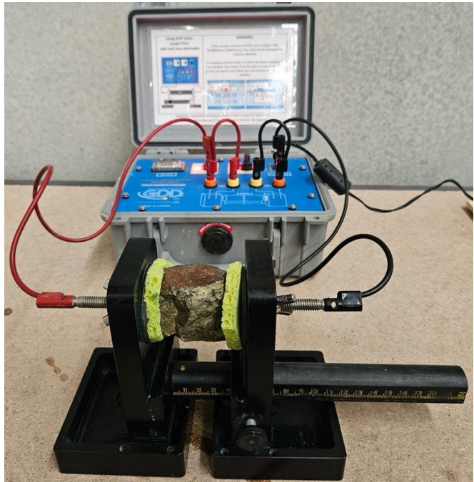
Figure 1: Prince Of Wales prospect sample RK008302 10.15% Cu and 65.8g/t Ag 2 , being tested for Induced Polarisation, chargeability, galvanic resistivity and inductive conductivity
