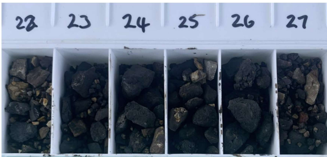
Figure 1: RC drill hole GRCD015 intercepted 21.30% Mn over 5 metres from 22m, including 2 metres at 29.65% Mn. Visible black manganese mineralisation in RC chip tray (compartments 28x24x45mm)
