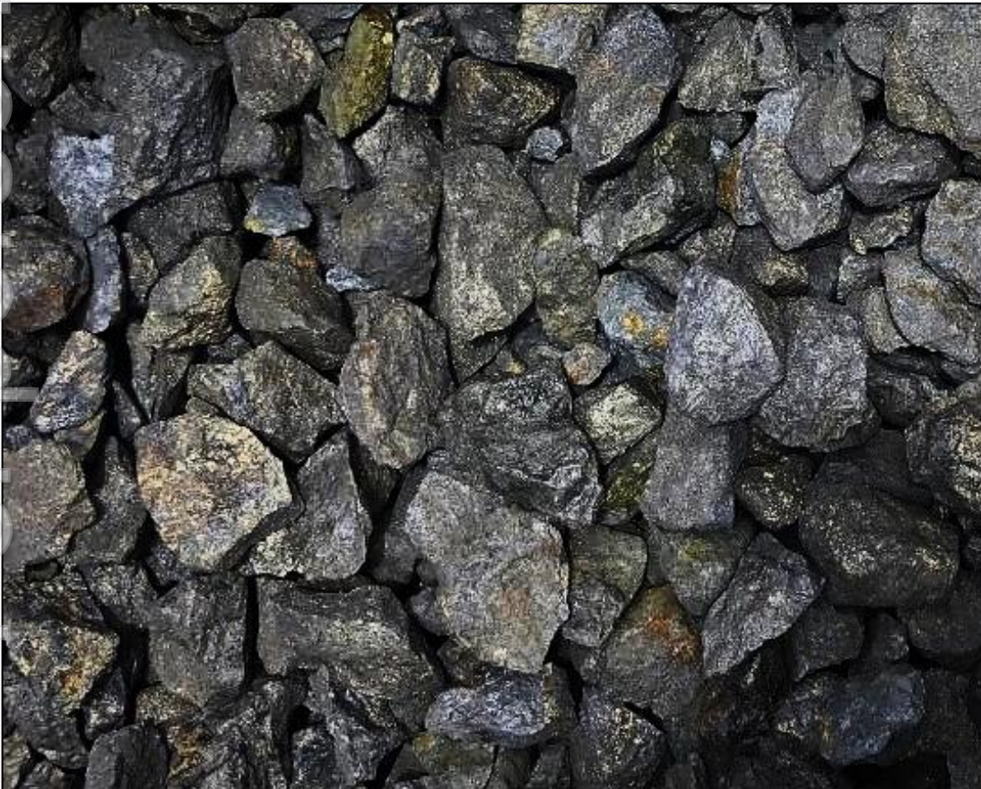
Photo 3. Mined and coarsely crushed Montezuma mineralisation. Representative sample assays of mineralisation only batches averaged 9.02% antimony (Sb), 769 g/t silver (Ag) and 15.47% lead (Pb)
