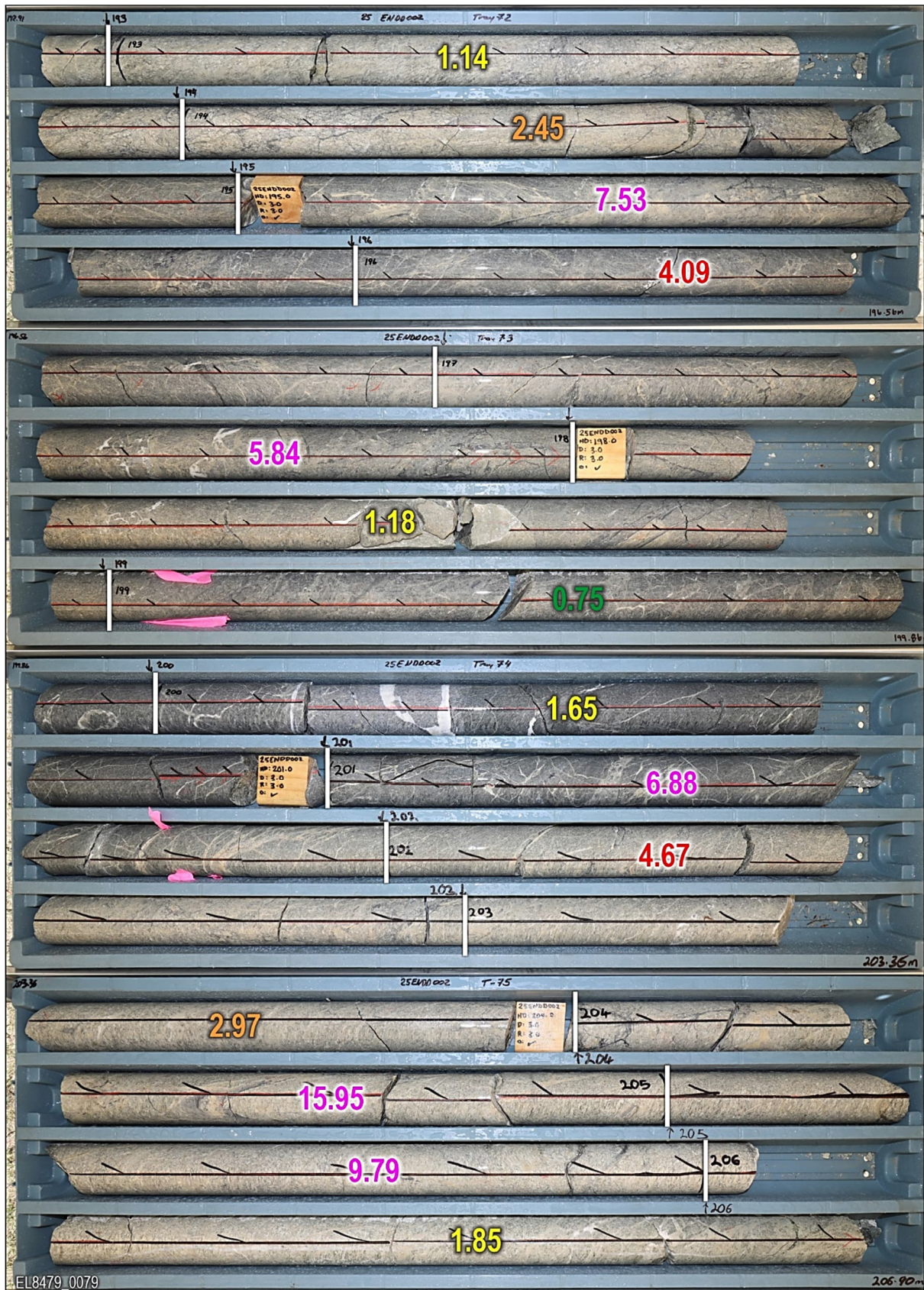
Photo 2. Core tray photos of 25EIDD002 interval 25m @ 5.23g/t Au from 194m. Distinctive paler coloured zones (silica-sericite altered) typically host better grades (although not exclusively) and are interpreted to have overprinted the darker coloured zones (propylitic/chlorite altered). The numbers superimposed on the core are the reported gold assay grades over each respective sample interval.
