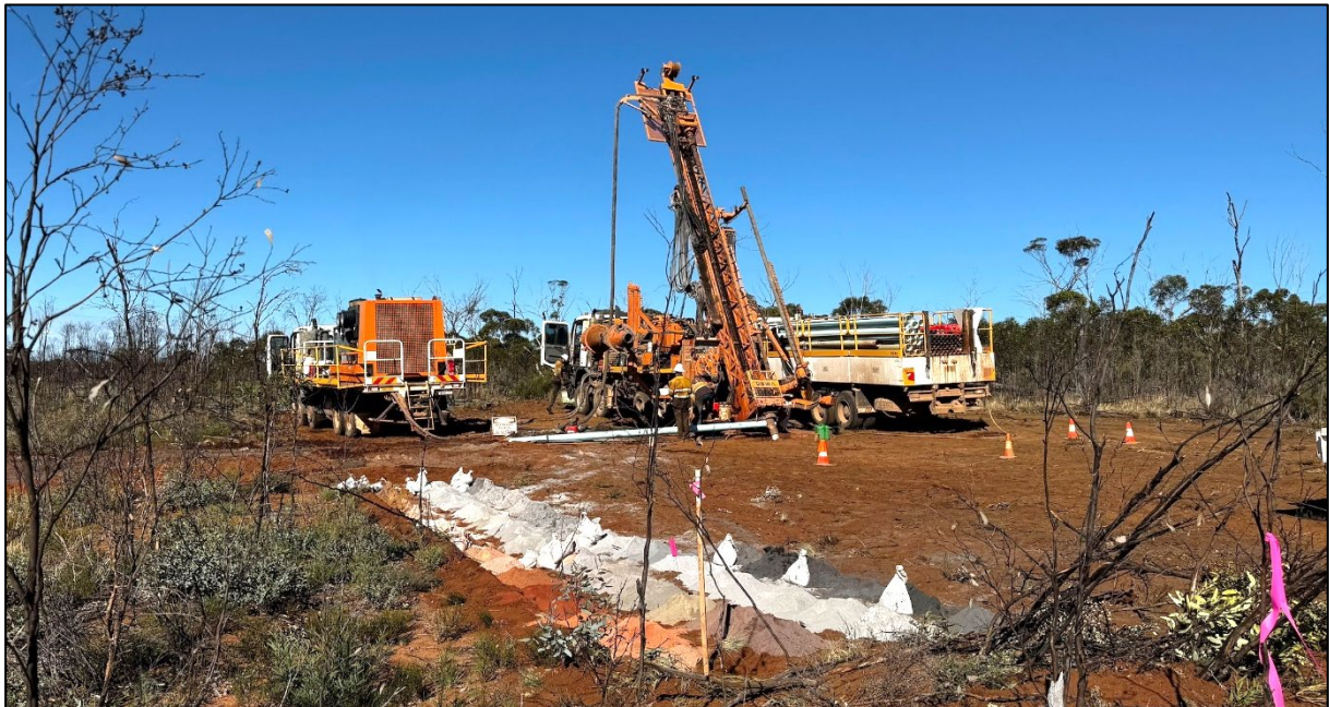
Figure 1: Balladonia Project: Reverse Circulation drilling underway on the first drill-hole
