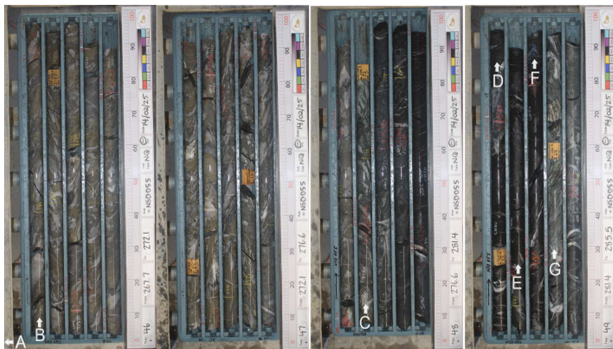
Figure 5 NSD055 276.7 - 285.5m A, Carbonaceous shales (3m up hole). B, weakly sericitised, silica-sulphide altered volcaniclastic. C, Sulphide-silica volcaniclastics. D, Pelite. E, Sulphide-silica volcaniclastics. F, Pelite. G, Basalt. The target horizon is C to end-F. No significant assays. Anomalous mineralisation 280-283.5m.
