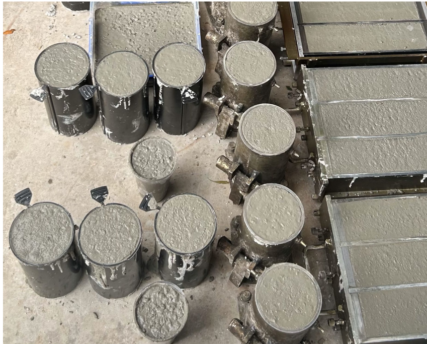
Figure 1 - Concrete sample preparation
