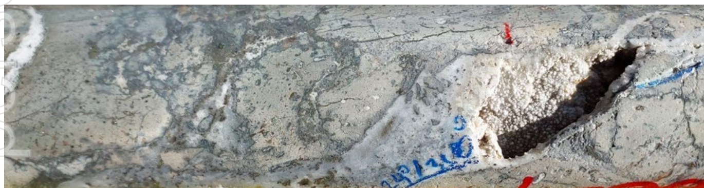
25VDD002_198.25-198.52m. From Sample No 386654, 198.25-198.67m (0.42m) 0.57 g/t Au, 5.28 g/t Ag. Mineralised chalcedonic vein breccias cemented by chalcedonic quartz with colloform and crustiform epithermal vein textures and abundant blebby pyrite, sphalerite and dark grey sulphide. 5% pyrite-sulphide. Within strongly silica-clay-altered basalt. Open spaces with drusy silica.
