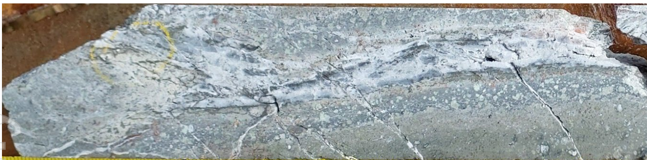
25VDD002_195.76-196.15m. From Sample No. 386651, 195.76-196.56m (0.8m) 11.4 g/t Au, 6.52 g/t Ag. Mineralised chalcedonic vein within strong clay-altered basalt. Colloform and crustiform epithermal vein textures, open spaces with drusy quartz. Blebby and disseminated pyrite, sphalerite and grey sulphide.
