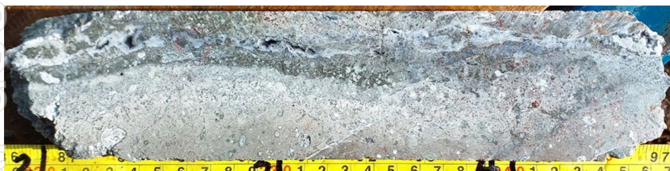
25VDD002_199.58-199.83m. From Sample No. 386656, 199.32-199.9m (0.58m), 26.4 g/t Au, 39.70 g/t Ag. Colloform banded and crustiform chalcedonic silica veins. Open spaces with drusy quartz. Blebby and fine pyrite, sphalerite and galena-tennantite-tetrahedrite. The host lithology is a vesicular basalt and silica-clay-altered. Disseminated and blebby pyrite halo to the veins.
