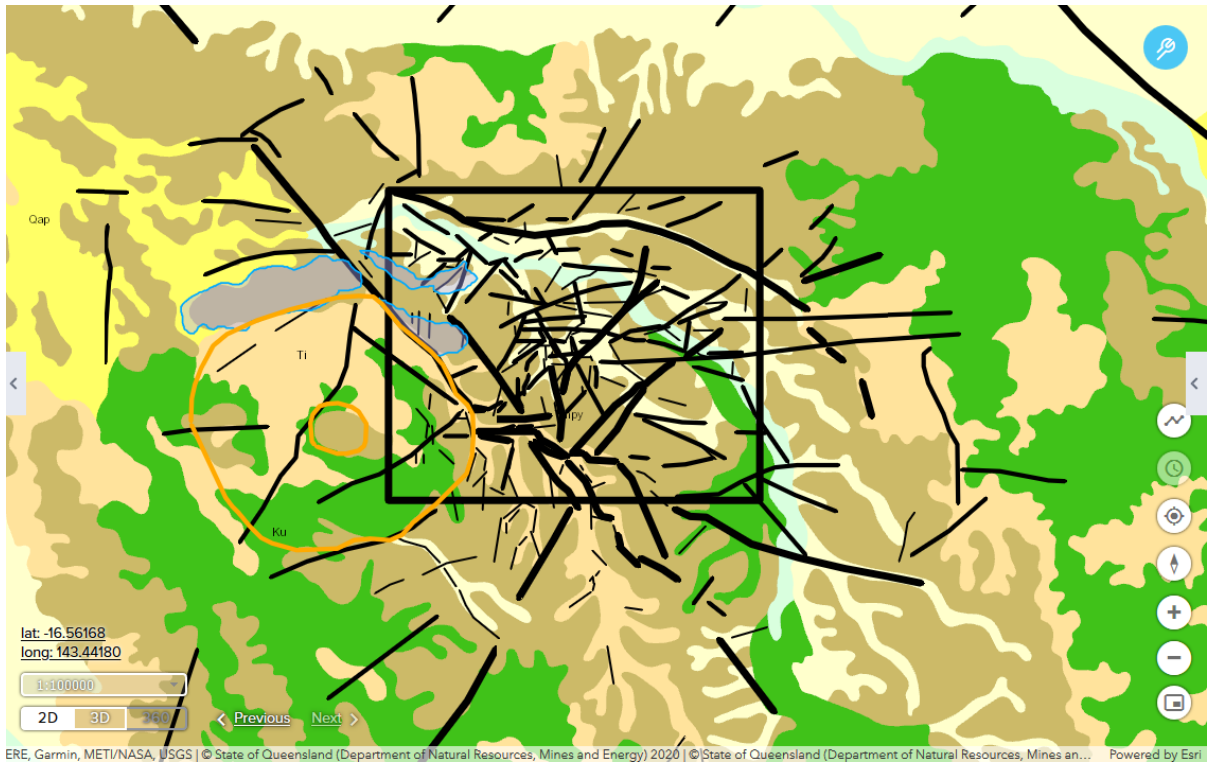
Figure 4. 1:100K GSQ Surface Geology. Overlain polygons (blue) represents mapped extents of outcropping felsic volcanic breccia and ignimbrite. Orange polylines represent sub-cropping (hypothesised) collapse cauldron with possible resurgent dome in centre. Black polylines are hypothesised sub-surface penetrative structures interpreted from combinations of remotely sensed data and field observations – particularly sub-surface influences on cover. The outcropping felsic volcanics may represent a partially exposed and structurally disrupted ring-dyke complex associated with collapse of the sub-circular feature. Landsat bands 7/6/2 and 5/6/2 highlight the outcrops and inferred sub-crops against the more extensive unconsolidated cover (Wyaaba beds and Bulimba formation) particularly well. (Source TRP).
