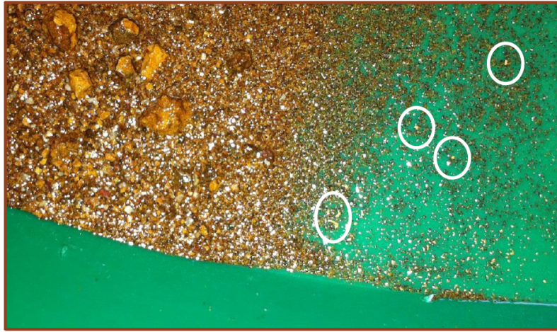
Figure 6. Crushed Iron pisolith sample containing gold grading up to 282 g/t in iron pisolites. (Source: TRP)
