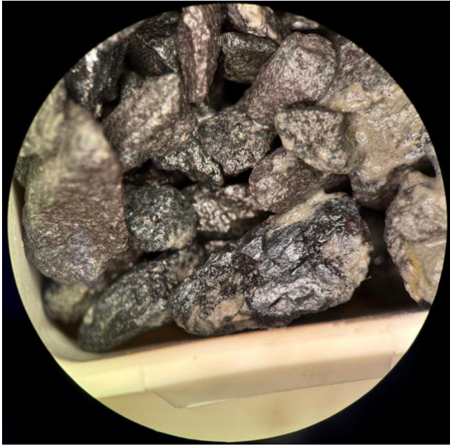
Figure 2. Chalcocite from DAN25005 between 27.43-28.96m depth.
