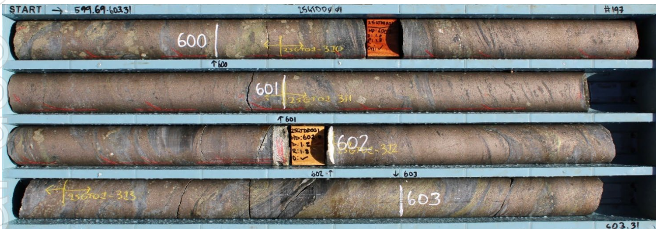
Figure 2: Massive and Blebby Sulphide intersection (599.69m – 603.31m shown) in Drill Hole 25GTDD001
