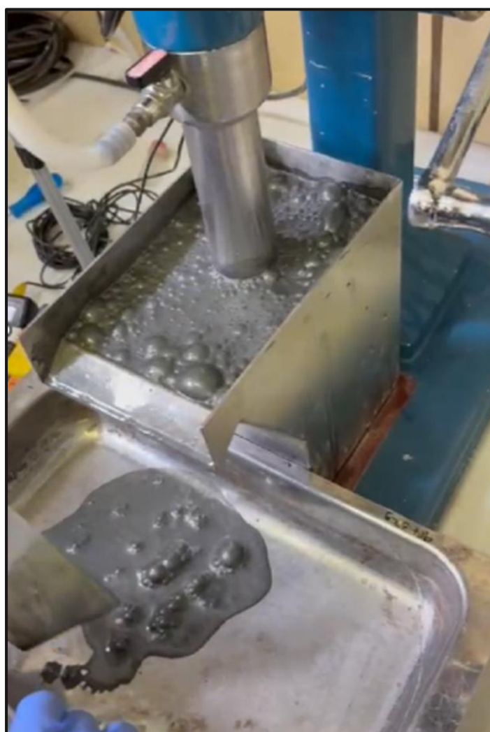
Figure 1: Flotation test producing high-value rougher concentrate
