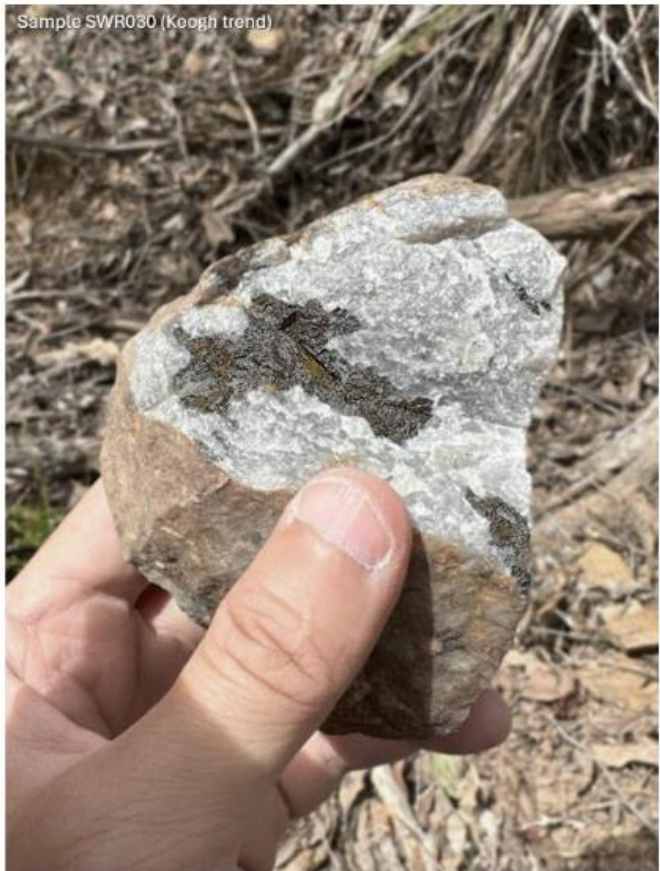
Figure 8. Large cassiterite (tin-oxide) dark mineral crystals and aggregates, from the Sweetwater area: L) Sample SWR029 (16.70% SnO 2 ) and R) Sample SWR030 (8.65% SnO 2 )
