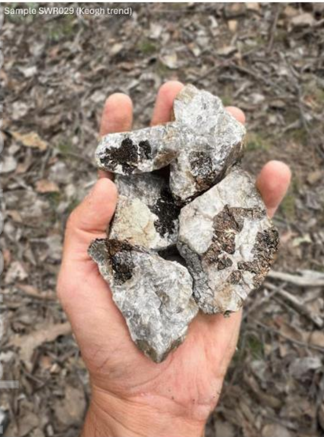
Figure 8. Large cassiterite (tin-oxide) dark mineral crystals and aggregates, from the Sweetwater area: L) Sample SWR029 (16.70% SnO 2 ) and R) Sample SWR030 (8.65% SnO 2 )
