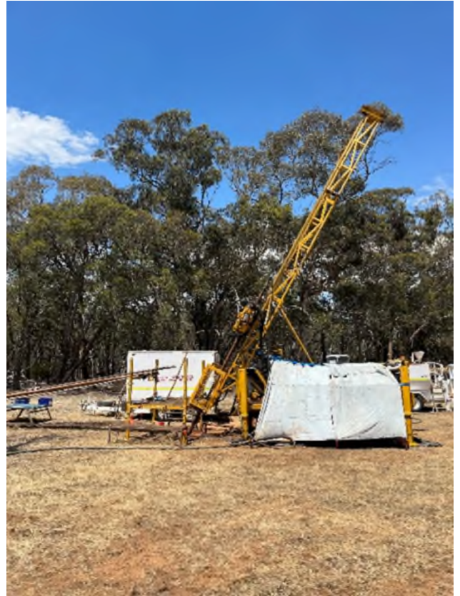
Figure 2 - Irvine Project (Stawell zone) - Diamond drill rig in operation with covering noise attenuation materials
