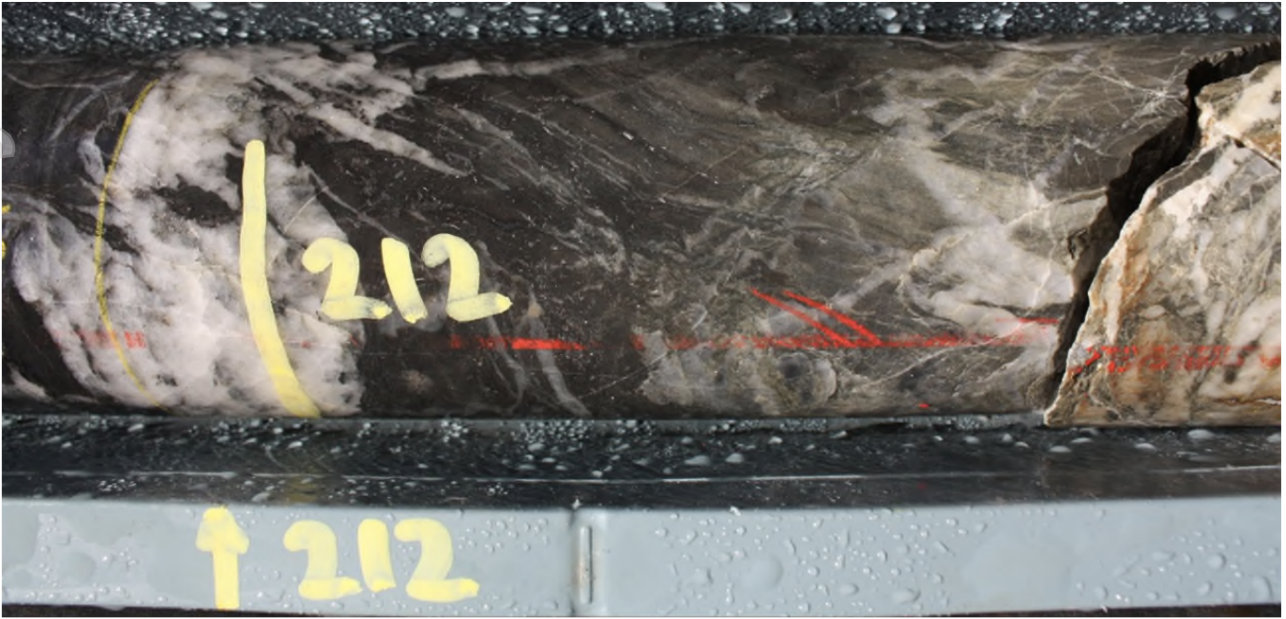
Figure 6 - RD045. 212.00 212.20m Acicular arsenopyrite needles developed adjacent to steeply inclined shear structure within overlying western sediments 9
