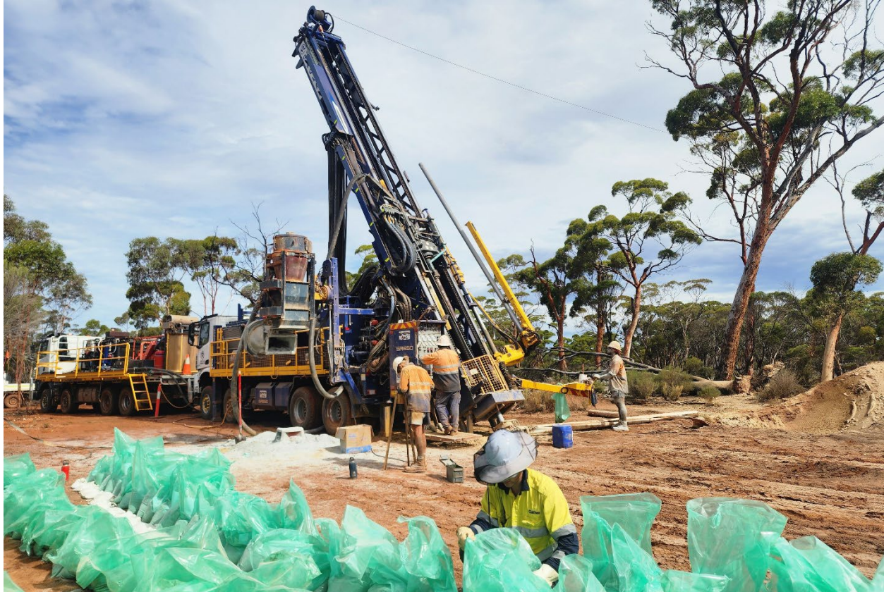
Figure 2. Reverse Circulation drilling at Cognac West prospect, March 2025
