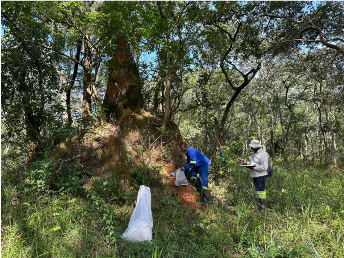
Figure 20. Termite hill geochemical sampling underway at Nyungu South Prospect
